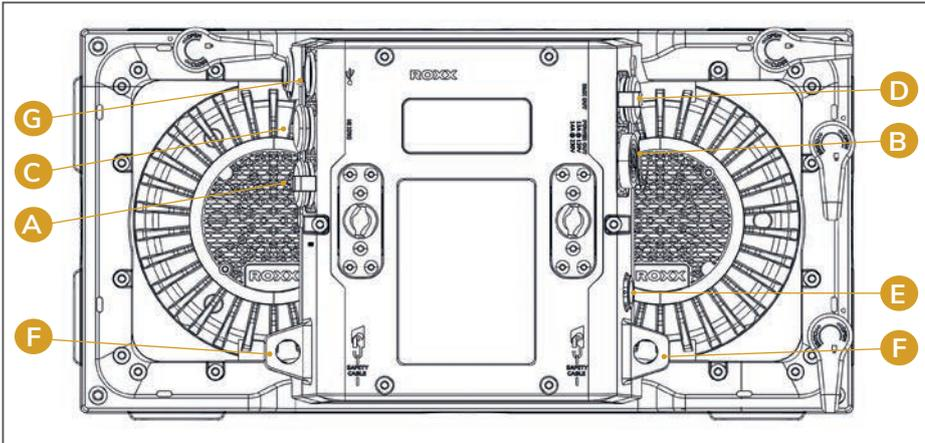
**A: Mains In:** IP65 Power input connector with rubber sealing cap. Connect using the provided power cable (when not in use, always close with rubber sealing cap).
