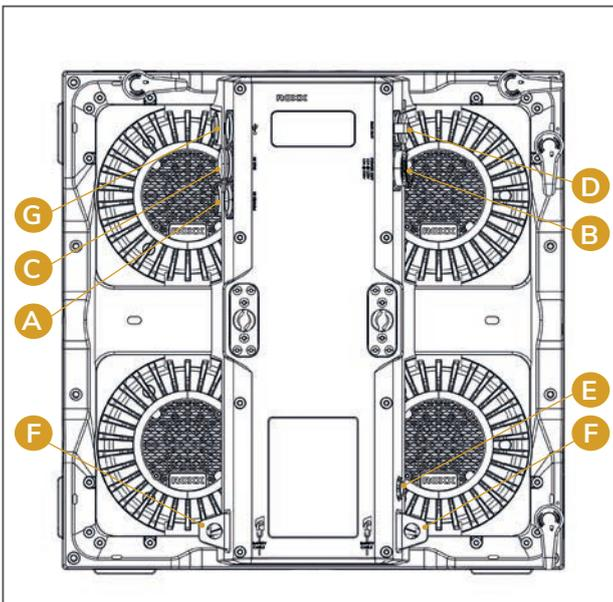
**A: Mains In:** IP65 Power input connector with rubber sealing cap. Connect using the provided power cable (when not in use, always close with rubber sealing cap).
