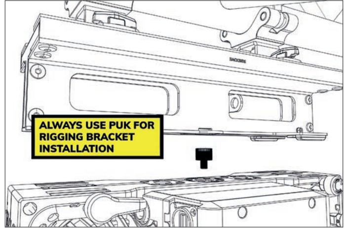
For seamless connection of multiple Blinders, to avoid gaps due to bracing of the truss structure by variable, sliding mounting positions.
