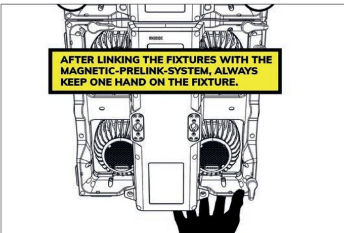
2. Pre-Link Magnets on top and side help to align the fixtures due cluster process and giving support operation for convenient and save interlocking.
