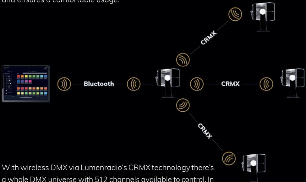
With wireless DMX via Lumenradio's CRMX technology there's a whole DMX universe with 512 channels available to control. In addition to ROXX® fixtures, devices from other manufacturers can also be controlled using integrated CRMX technology.
